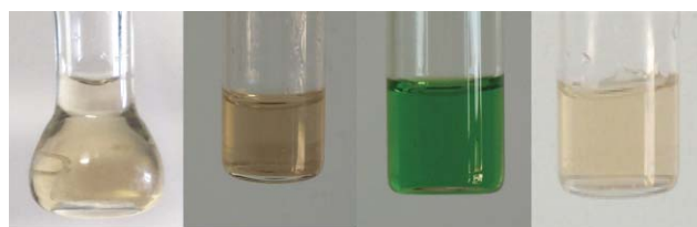
Fig. 1 From left to right: pure [HePy][Tf 2 N] and its solution with [Al][Tf 2 N] 3 , [Ni][Tf 2 N] 2 and Y[Tf 2 N] 3 .
